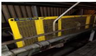
Guards for conveyor motor and belt to prevent human manipulation of counting system
