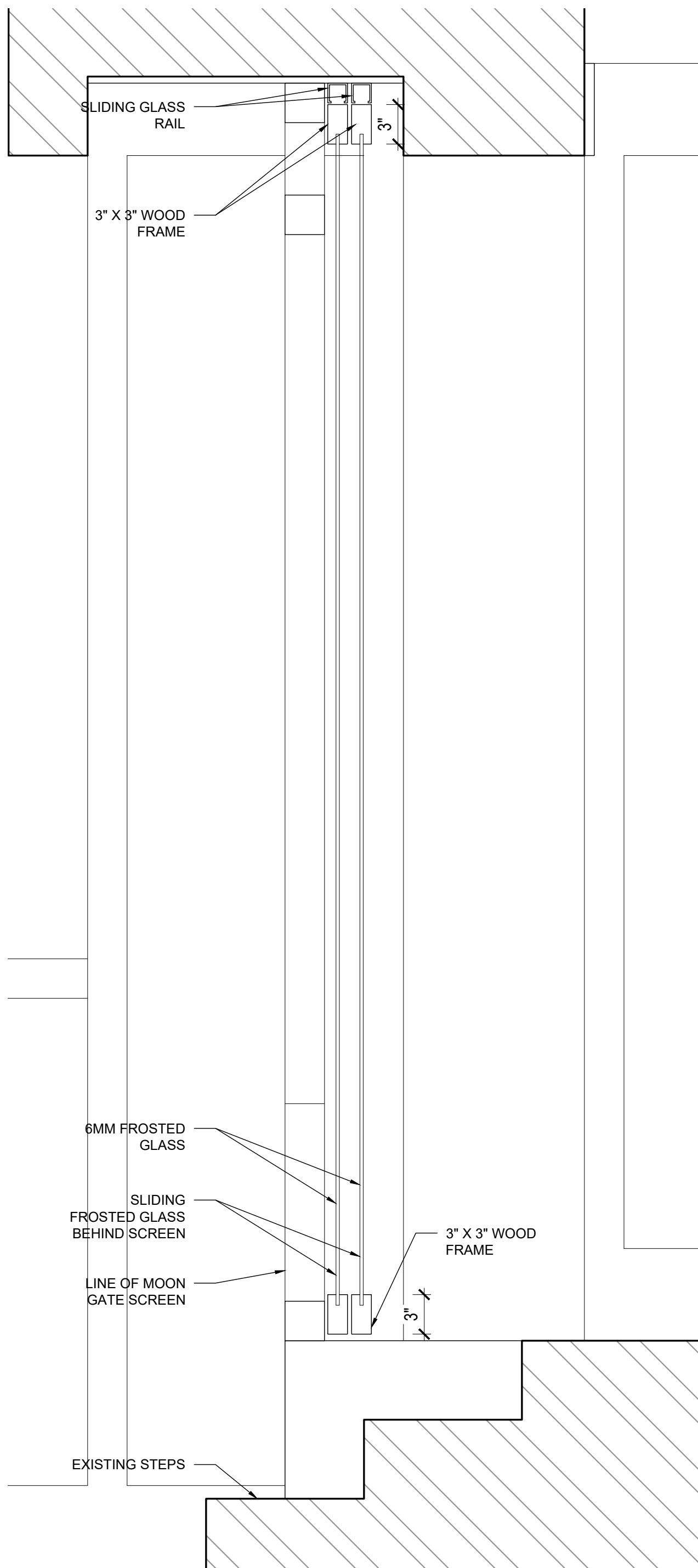
SLIDING SCREEN SECTION
