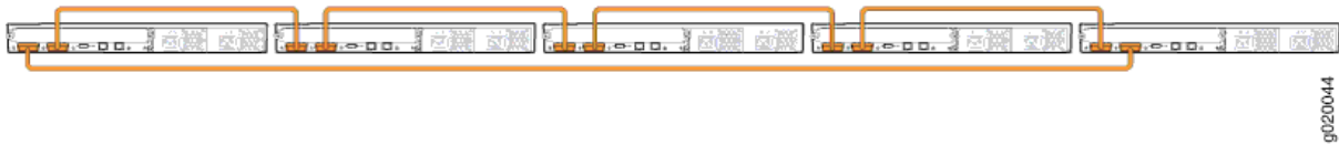
Figure 7. Adjacent Racks - Ring Topology with long cables
